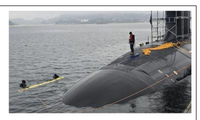
recovery of a UUV via submarine torpedo tube with the REMUS 600 UUV also built by HII.
